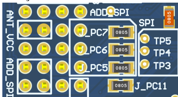
Figure 5.3: Additional GPIO and SPI channel.
