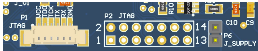
Figure 3.7: Programmer (P1 and P2) and jumper (P6) connectors.
